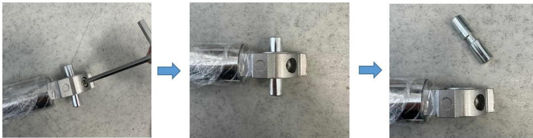
Figure 5-4 Remove Fixing Stud
